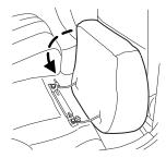
**WARNING:** Make sure safety belt buckle heads are through elastic holders on seat backs. Safety belt buckles may break if they are trapped underneath the seatback as the seatback is rotated down.
